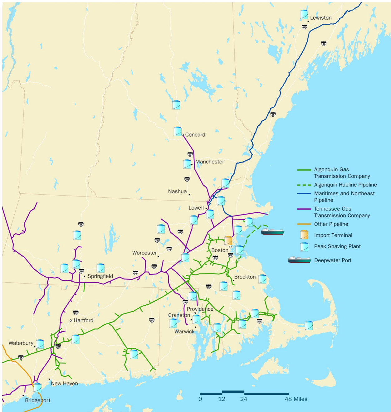
Figure 6. Pipeline and LNG Infrastructure in New England
